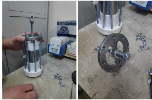
Figure 5. Casting holder a) setup for casting; b) stabilizer
