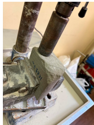
Figure 2. Drilling the core plug perpendicular to the bedding
