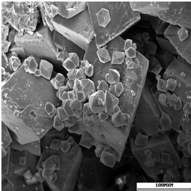
**Figure 6. Quartz crystals on the dolomite crystals from well A-61 at 3424 m, Middle Carboniferous, Lower Moscovian Substage (C<sub>2</sub>m<sub>1</sub>) (JEOL T-100 scanning electron microscope)**
