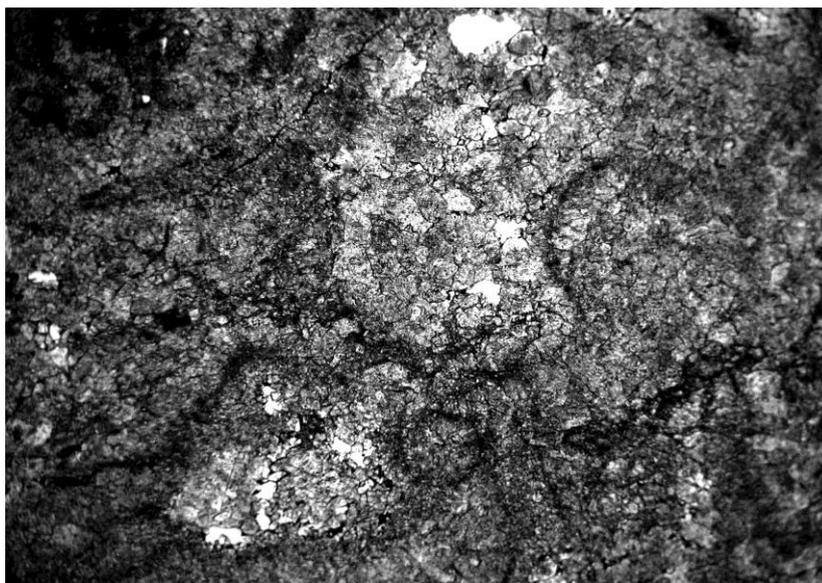
Figure 2. Lace-form thin section of the Tortkol field, well No.8, int. 3493-3501 m, 40x
