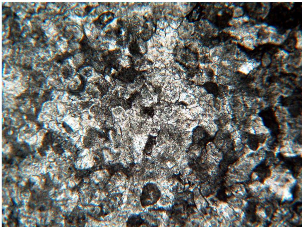
Figure 3. Thin section, 25x magnification, *Donezella* bufflstone, well U-2, int. 3958 m
