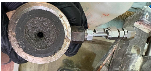
Figure 16. Core sample with a 3 mm diameter channel drilled halfway into the core
