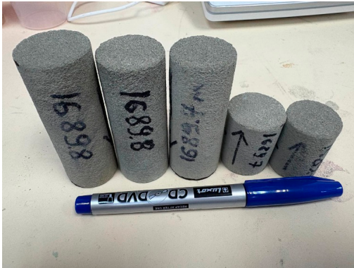
Figure 3. Sandstone core plugs after being machined using a standard lathe
