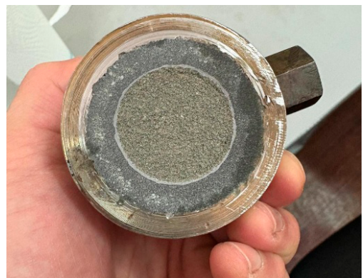
Figure 6. Core before and after facing off by using a standard lathe in the machine shop a) before; b) after
