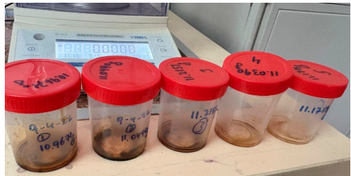
Figure 9. Polyethylene test bottles used to collect effluent from the core
